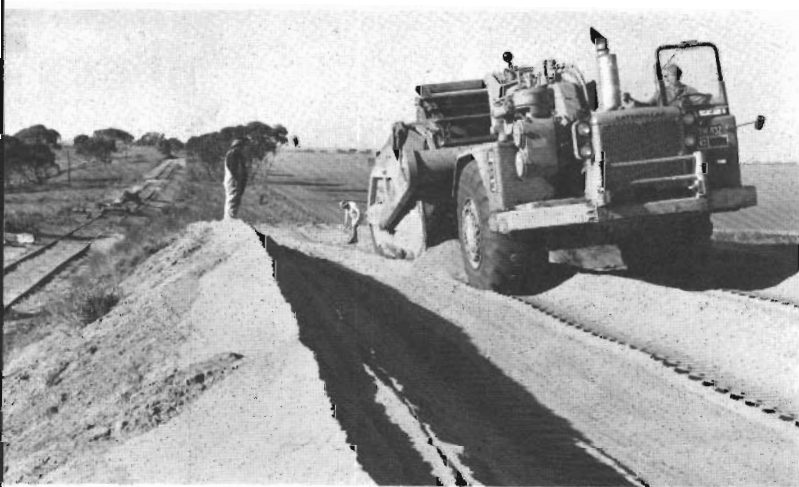
A modern earthmover levels a Mallee sand dune in a few hours, preparatory to planting with cereal rye to stabilise the light, sandy soil.
